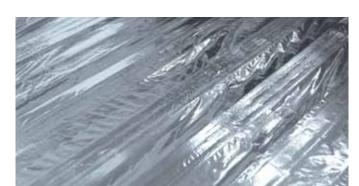
Vapour barrier consists of bitumen membrane covered with aluminium foil. This membrane is intended for application on the metal profiled decking as the vapour barrier layer of the roofing system.
