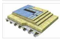
Flat roof structure with bitumen membrane.
