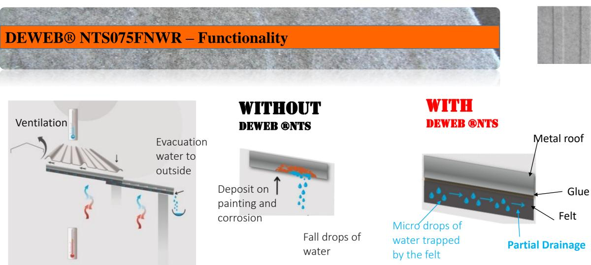
DEWEB<sup>®</sup> NTS075FNWR has a high absorption capacity with a quick absorption time and a low raising of water by capillarity, few centimeters, from bottom of slope.
