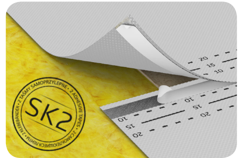
To gain proper sealing of overlaps, use the line which is 10 cm from the membranes edge
