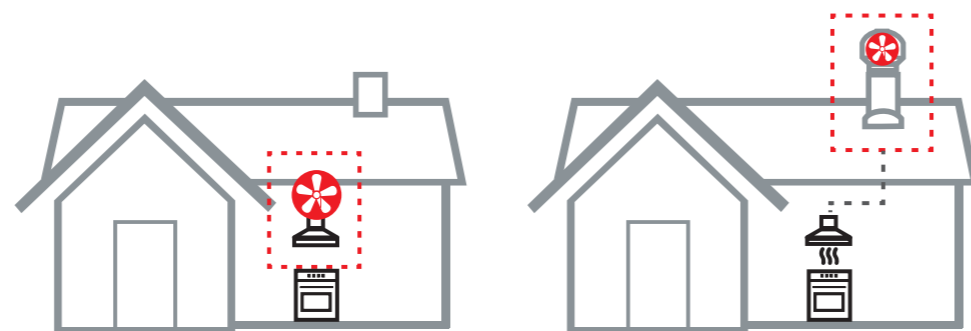
Kitchen extractor hood – traditional solution
