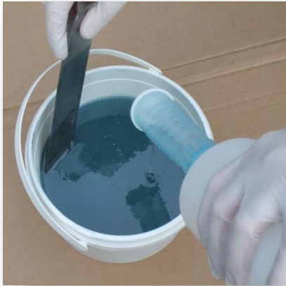
Measured and decanted catalyst is added to the resin
